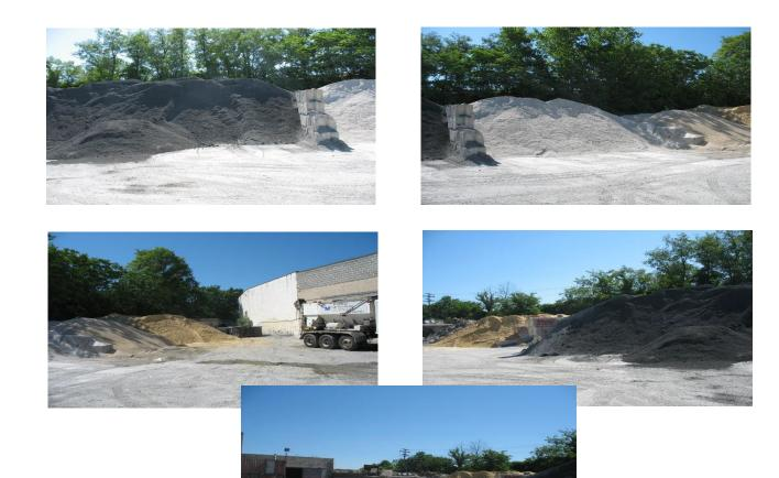
Operations for the concrete batching plant will also utilize the components used to make the concrete or cinder blocks shown above, except more cement and more water is required to make ready-mix concrete. The components will be placed into barrels attached to trucks, water is added and then the cycle mixer in the barrels are activated to keep the concrete from hardening—all on the same site.
