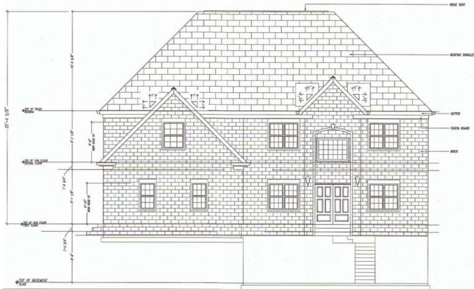
1. FRONT ELEVATION SCALE: \frac{3}{8}" = 1'-0" (FULLY DIMENSIONED)
