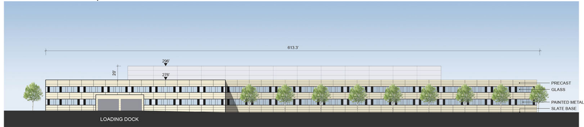
03 | OFFICE BUILDING - NORTH ELEVATION
