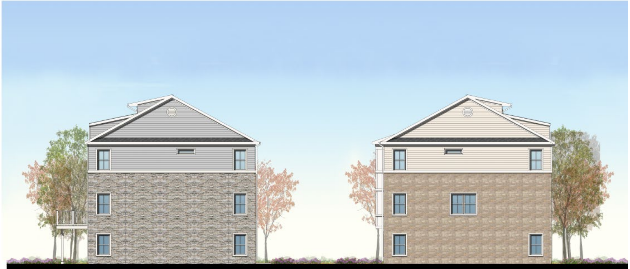
LEFT SIDE ELEVATION LOT 1 STONE: NEW ENGLAND LEDGESTONE HORIZ. SIDING: PLATINUM GRAY
