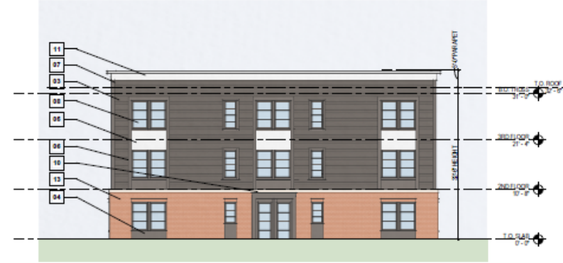
BUILDING 3.3 - REAR ELEVATION
