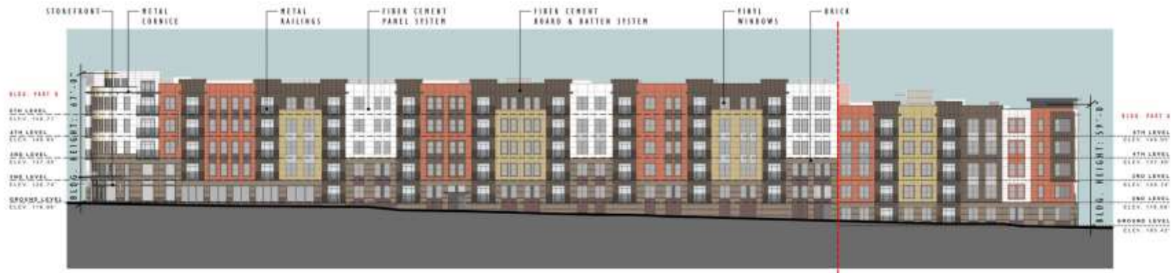
1. EASTWEST HIGHWAY ELEVATION
