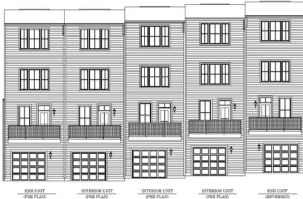
Rear Elevation 1 - Building F 1/4" = 1'-0"
