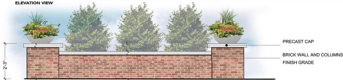
SEAT WALL ELEVATION VIEW
