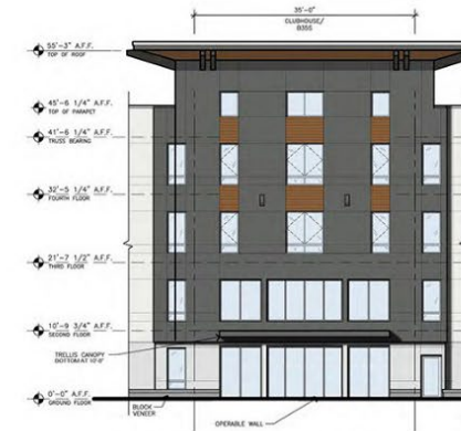
9 Building 1 - East Elevation - Inside SCALE: 1/8" = 1'-0"
