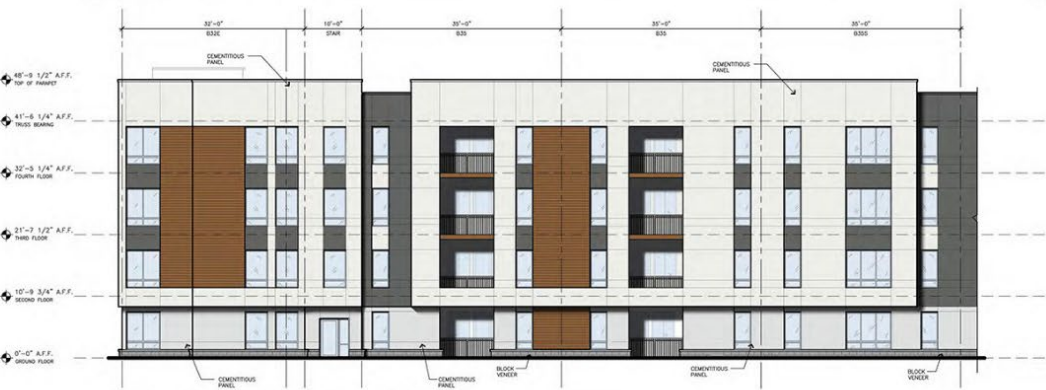
8 Building 1 - Northeast Elevation - Inside SCALE: 1/8" = 1'-0"
