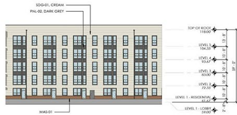
③ NORTH COURTYARD - SOUTH ELEVATION SCALE: 1" = 20' 0"
