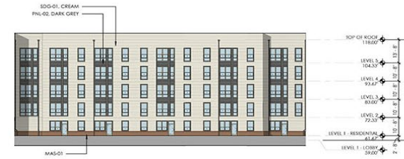
④ NORTH COURTYARD - EAST ELEVATION SCALE: 1" = 20' 0"
