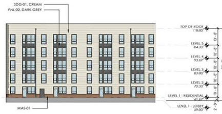
⑤ SOUTH COURTYARD - SOUTH ELEVATION SCALE: 1" = 20' 0"
