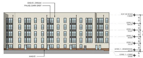
② NORTH COURTYARD - WEST ELEVATION SCALE: 1" = 20' 0"
