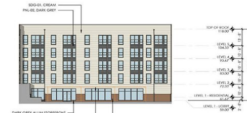
① NORTH COURTYARD - NORTH ELEVATION SCALE: 1" = 20' 0"
