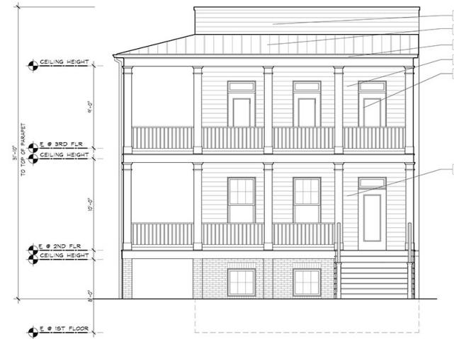
1 FRONT ELEVATION - 2-STORY PORCH A2.5 1/4" = 1'-0"
