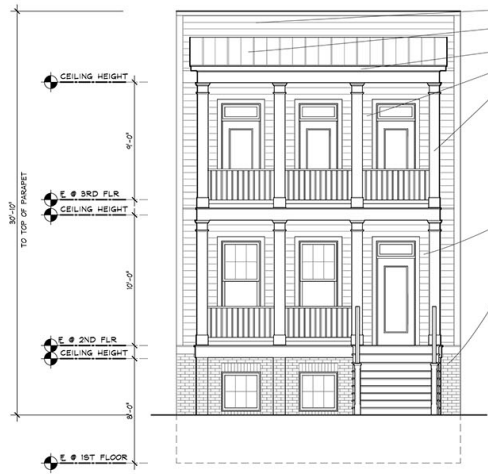
1 FRONT ELEVATION - 2-STORY PORCH A2.6 1/4" = 1'-0"
