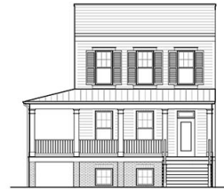
2 FRONT ELEVATION - 1-STORY PORCH A2.5 1/4" = 1'-0"
