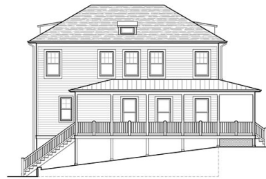
2 SIDE ELEVATION A2.1 1/4" = 1'-0"
