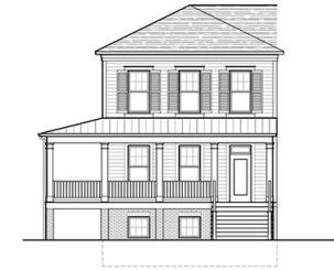
2 FRONT ELEVATION - 1-STORY PORCH A2.5 1/4" = 1'-0"
