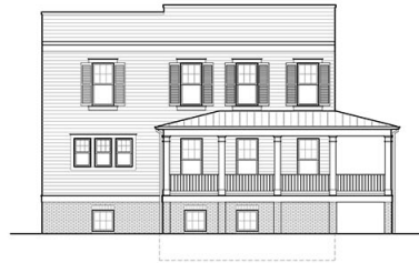
4 SIDE ELEVATION - 1-STORY PORCH A2.5 1/8" = 1'-0"
