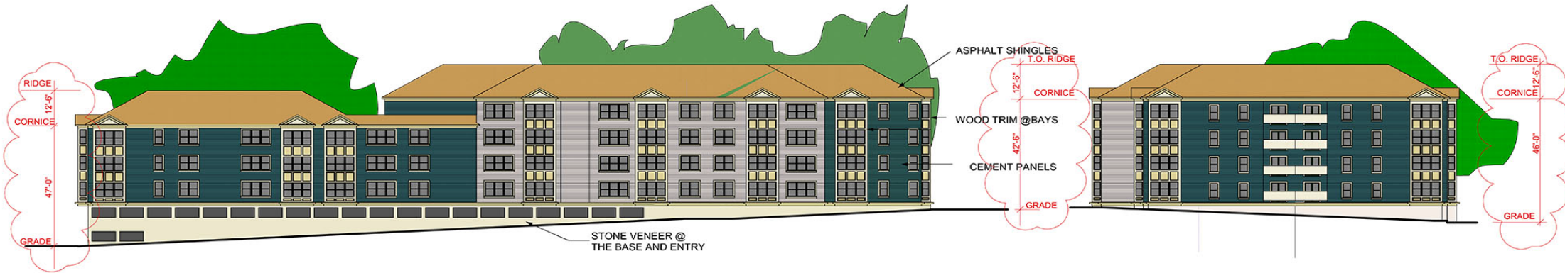
REAR ELEVATION BUILDING 2 SCALE : 1/16" = 1'-0"
