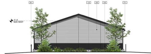
4 GARAGE 1000 - SOUTH ELEVATION 3/16" = 1'-0"
