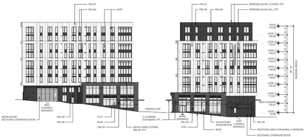
② SOUTH ELEVATION SCALE: 1" = 20'-0"
