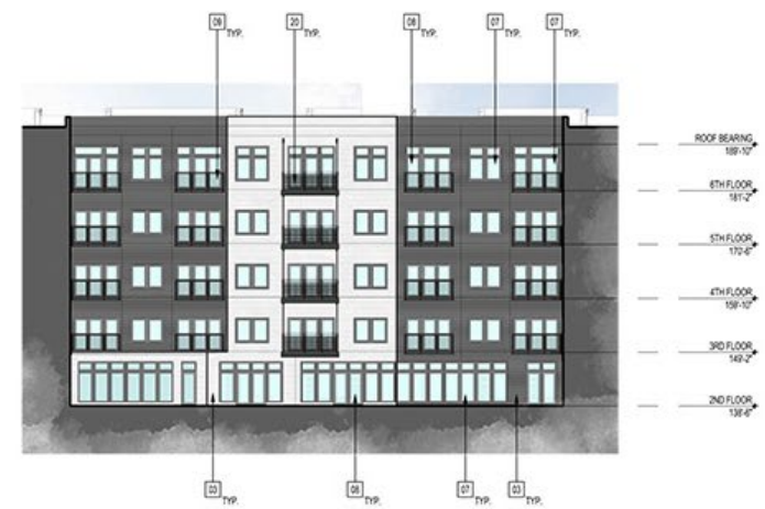
4 WEST COURTYARD ELEVATION Scale: 1/16" = 1'-0"
