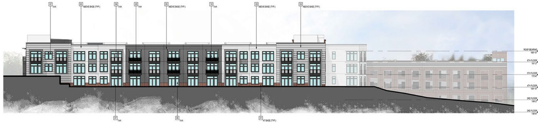
1 SOUTH-EAST ELEVATION @ REAR UNITS Scale: 3/16" = 1'-0"
