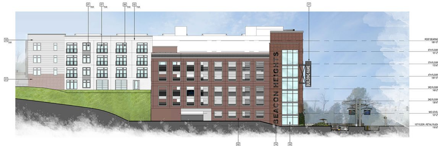
2 NORTH-EAST ELEVATION @ PRECAST GARAGE Scale: 3/16" = 1'-0"
