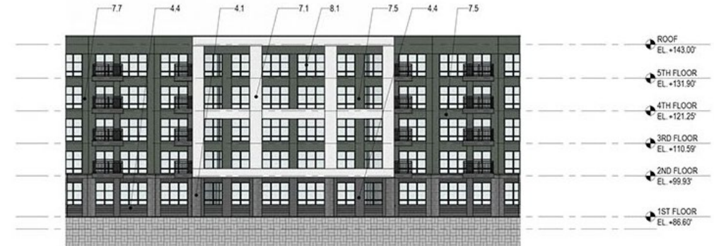
3 COURTYARD ELEVATION - NORTH SCALE: 1/16" = 1'-0"
