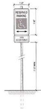
LEGEND & BORDER - RED BACKGROUND - WHITE NOTE: APPROPRIATE ARCH PLATE MAY BE USED WHEN IT IS NECESSARY TO IDENTIFY LOCATION OF HANDICAPPED PARKING AND ACCESS AISLE HANDICAPPED PARKING AND ACCESS AISLE SIGN NTS
