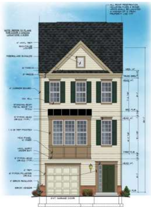
1 FRONT ELEVATION C. W. BRICK WATERBURY
