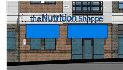
ENLARGED RETAIL SIGNAGE ELEVATION 1/4"=1'-0"
