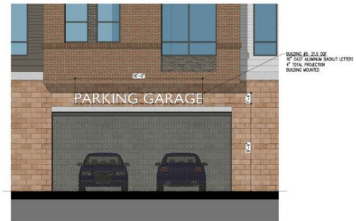
ENLARGED PARKING SIGNAGE ELEVATION 1/4"=1'-0"
