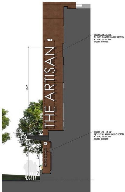
ENLARGED BUILDING SIGNAGE ELEVATION 1/4"=1'-0"
