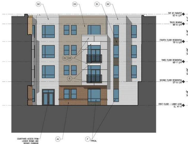
NORTH COURTYARD ELEVATION 1/8"=1'-0"
