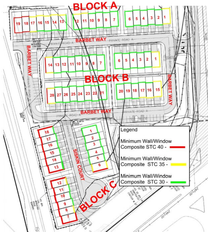
Figure 7: Minimum wall/window composite requirements
