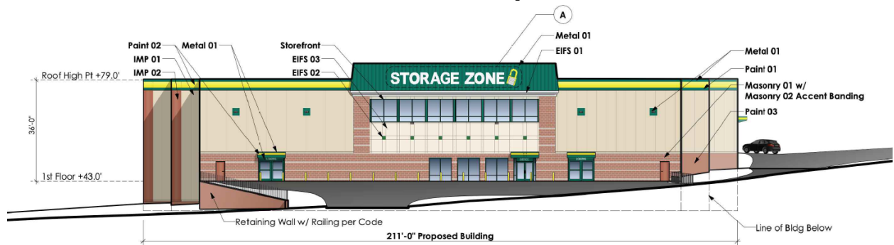
Figure 2: Northwest Architectural Elevation
