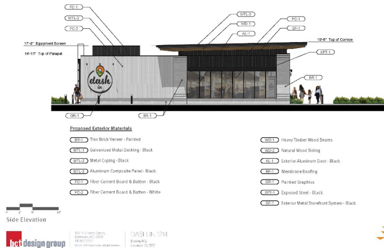
Figure 4: Side Elevation (Facing South) of the Food or Beverage Store
