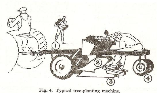
(1) Rolling coulter. (2) Double mouldboard plow or middle buster. Not essential in the absence of heavy ground cover. (3) Planting shoe, which opens the trench. (4) Packing wheels, which close trench and firm the soil.
