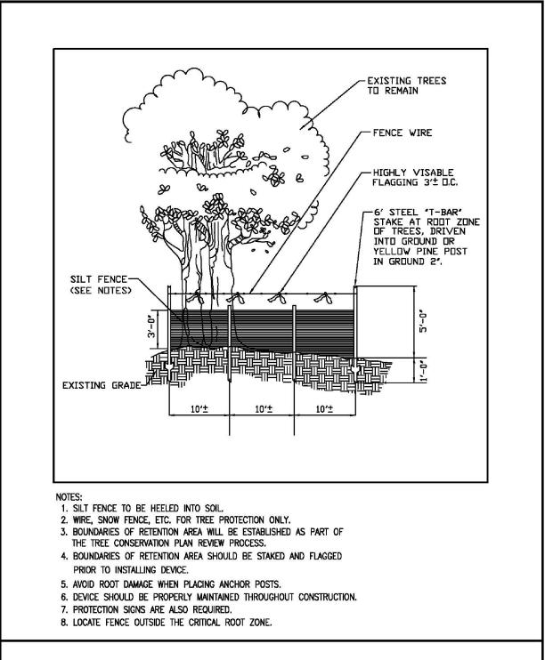
TYPE 4 (TEMPORARY) TREE PROTECTION FENCE COMBINATION SILT FENCE & TREE PROTECTION
