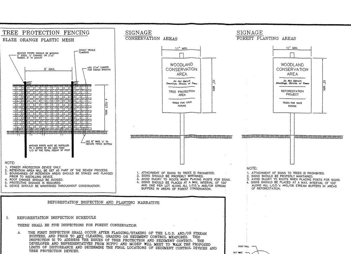
THE SECOND INSPECTION SHALL OCCUR AFTER PLACEMENT OF SEDIMENT CONTROL DEVICES AND/OTE: TREE PROTECTION DEVICES, AND PRIOR TO CLEARING AND GRADING. THIS INSPECTION IS TO
