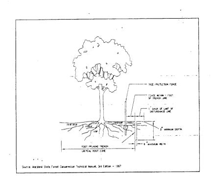
1. RETENTION AREAS TO BE ESTABLISHED AS PART OF THE FOREST CONSERVATION 2. BOUNDARIES OF RETENTION AREAS SHOULD BE-STAKED; FLAGGED AND/OR FENCED PRIOR TO TRENCHING. 4. TRENCH SHOULD BE IMMEDIALTEY BACKFILLED WITH SOIL REMOVED OR OTHER HIGH 5. ROOTS SHOULD BE CLEANLY CUT USING VIBRATORY KNIFE OR OTHER ACCEPTABLE
