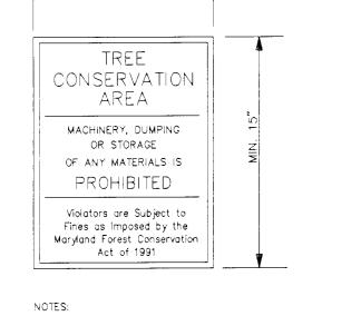
SIGN TO BE LAMINATED CARDBOARD OR PLASTIC WHITE WITH RED PRINT. 2. BOTTOM OF SIGNS TO BE HIGHER THAN TOP OF TREE PROTECTION FENCE. 3. TREE CONSERVATION AREA SIGNS WILL BE SECURELY ATTACHED TO AT LEAST EVERY FIFTH POST AND SHALL REMAIN IN PLACE IN PERPETUITY. TREE CONSERVATION SIGN
