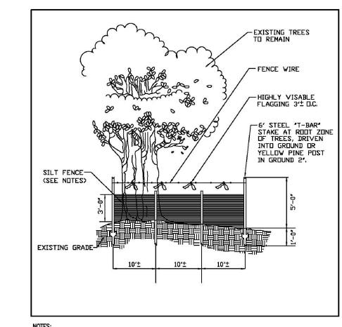
SILT FENCE TO BE HEELED INTO SOIL.
