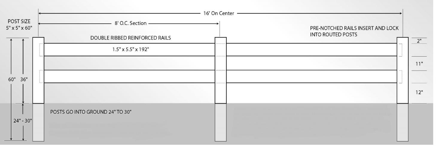
Boundary Fence (Future Installation) and Permenant Protective Fence (Installed with Afforestation)
