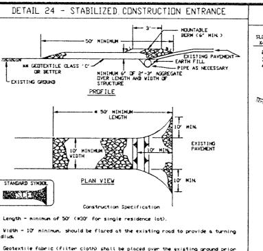
Length - minimum of 50' (#30' for single residence lot) 2. Vidth - 10' minimum, should be flared at the existing road to provide a turning residences to use geotextile. 4. Stone - crushed aggregate (2" to 3") or reclained or recycled concrete 5. Surface Vater - all surface water flowing to or diverted toward construction entrances shall be piped through the entrance, maintaining positive drainage. Pipe installed through the stabilized construction entrance shall be protected with a
